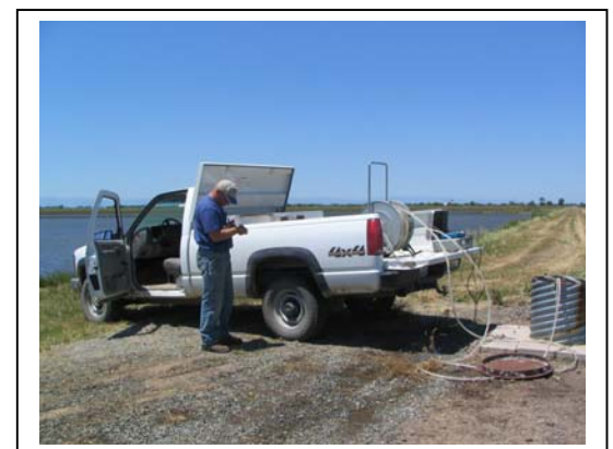
Figure 6. Groundwater quality sampling and monitoring at a dedicated monitoring well in Butte County.
