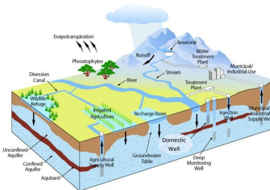
Also shown in Figure 1 are generalized depictions of an unconfined aquifer, a confined aquifer, and an aquitard.
